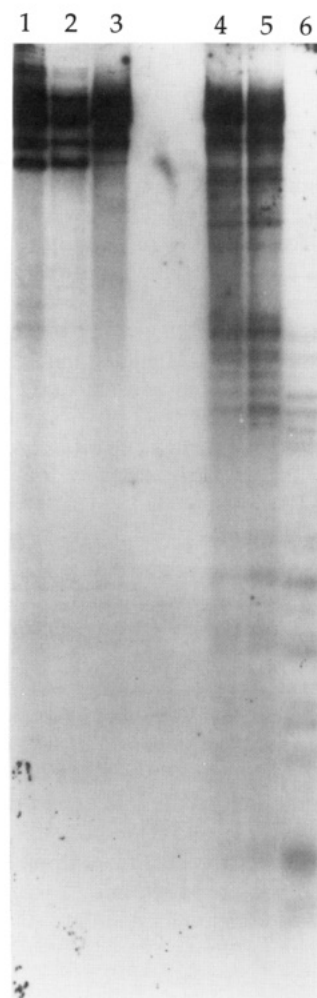
FIGURE 4: Polyacrylamide gel of pBR322 DNA, digested with Cl a1 and Eco R1 and end labeled as described in Materials and Methods. Lane 1: Unirradiated DNA. Lane 2: 150 \mu M DNA, irradiated with 4.56 J/cm 2 of 488-nm light. Lane 3: 150 \mu M DNA, 20 \mu M EB, and 210 \mu M MV, unirradiated. Lanes 4 and 5: Same as lane 3 but irradiated at 488 nm at fluences of 2.28 and 4.56 J/cm 2 , respectively. Lane 6: Unirradiated DNA, cleaved at guanines according to the Maxam–Gilbert method.
